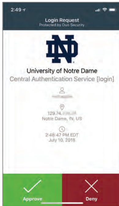
FIGURE 12.1 Smartphone-based multifactor authentication
