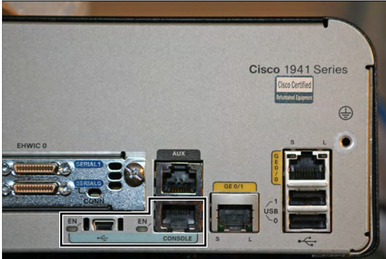
Figure 4-2 Different Console Port Connections
