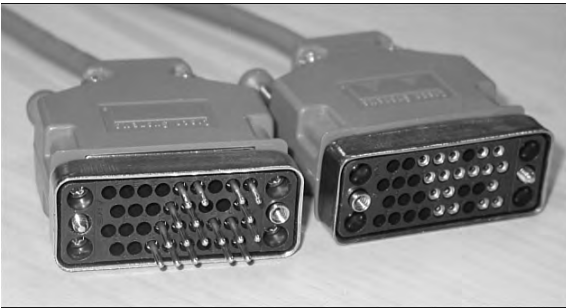
Figure 4-6 V.35 DTE and DCE Cables
