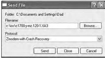
Figure 26-2 Sending the Cisco IOS Software Image File to the Router
