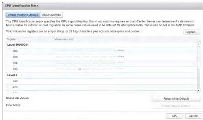
FIGURE 12.10 The CPU Identification Mask dialog box allows you to create custom CPU masks.
