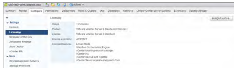
FIGURE 3.35 Licensing vCenter Server is managed through the vCenter Server Settings dialog box.
