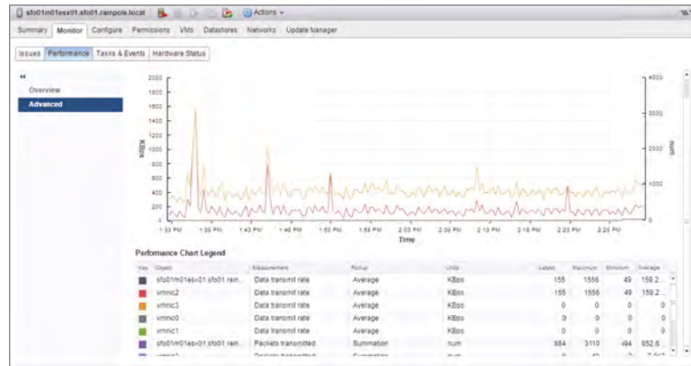
FIGURE 13.18 Packet rate and data rate can be overlaid on the same chart.
