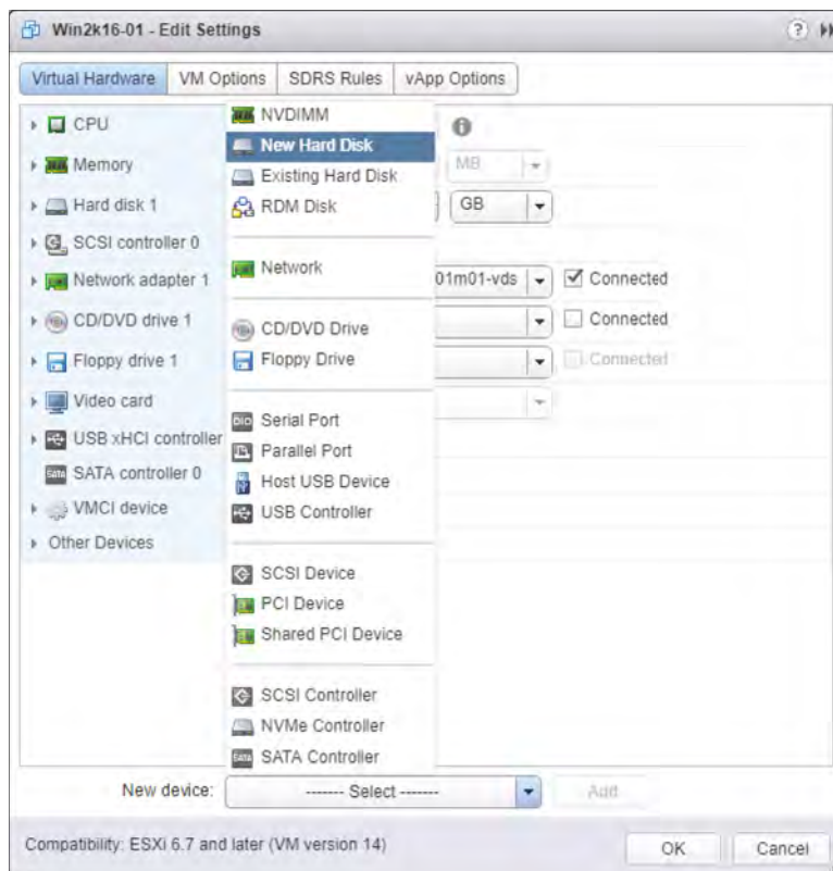
FIGURE 9.26 Users can add some types of hardware while the VM is powered on. If virtual hardware cannot be added while the VM is powered on, the operation will fail.
